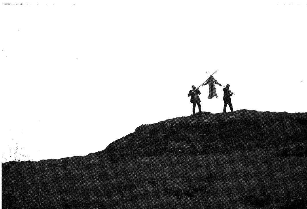
FIG. 1. Close-up view of Mid Hill foresight (with signal for identification from Brogar).
